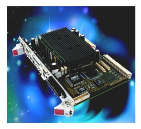
The VP7 VMEbus all-in-one 6U single board computer is designed to meet the needs of embedded application developers addressing markets like telecommunication (high bandwidth, broadband data or intelligent network switching), industrial automation, military and aerospace, medical, scientific, and imaging. Supported operating systems are Windows NT, Windows 98, MS-DOS, QNX, VxWorks, Solaris and others.
